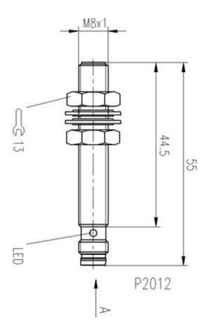
Inductive Sensors BES 516-343-S49-C M8x1 x 55 normally-open Sn=1,5mm shielded
